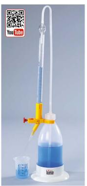
Burette with Schellbach stripes type Schilling / Burkle with original Burkle dosing armature.
