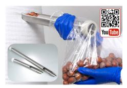
Sampler for pourable bulk goods up to approx. 1 cm (0.39 in.) in diameter. Corresponds to ISTA standard for seed lengths of 10 mm (0.39 in.) (wheat, oats) and 5 mm (0.20 in.) (flax, vetches).
