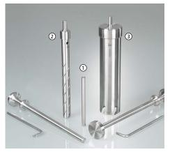
Meat sampler for microbiological sampling of carcass surfaces. The samplers for carcass sampling are similar to a cork drill. They can be used in the punch process (a destructive process, also called the cork drill or excision process) to remove a circular sample of tissue of 5 cm<sup>2</sup> (0.76 in<sup>2</sup>) from the surface. After the punch sample is cut out, it is removed from the carcass with a scalpel and tweezers.
