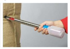
The core sampler is particularly suitable in the event that bulk goods are taken directly from sacks or bags and have to be filled into the original sampling bottle directly. QuickPicker is delivered complete with two 250 ml (8.45 oz.) PE sample bottles and with a cleaning brush. Corresponds to ISTA standard for seed lengths of 10 mm (0.39 in.) (wheat, oats) and 5 mm (0.20 in.) (flax, vetches).
