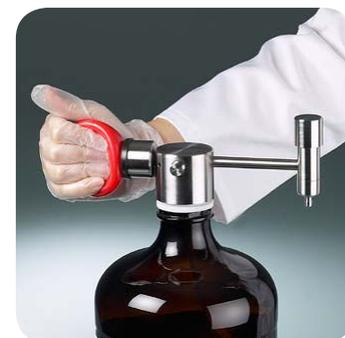
An excess pressure is built up in the container with the pump ball, forcing the liquid outward.
