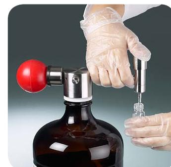
The self-closing discharge (with auto-stop function) of the Mini solvent pump ensures absolutely precise filling with no dripping at all.
